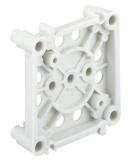
Blank base, base for supporting IBT boxes and boxes in opposing formwork in conjunction with support spars, can be combined via snap-in connection, if fitting the blank base using nails, magnet, adhesive, the fixing points must be plastered subsequently, for fitting:
